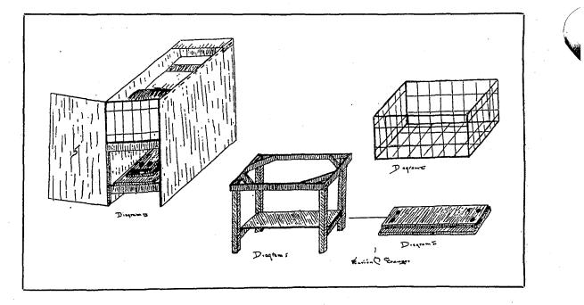
diagram II. The latter consists of two boards with a three-quarter inch space between to permit proper wiring for lights. The lower board is eighteen inches long, five and a half inches wide and three-quarters of an inch thick. The upper board is eighteen inches long, three and a half inches wide and one inch thick. Four sixty watt electric light globes are attached to this board with wiring for connection to electric current.
